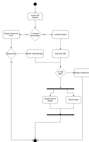
Fig. 3 Activity Diagram for Make Sabil Transaction
