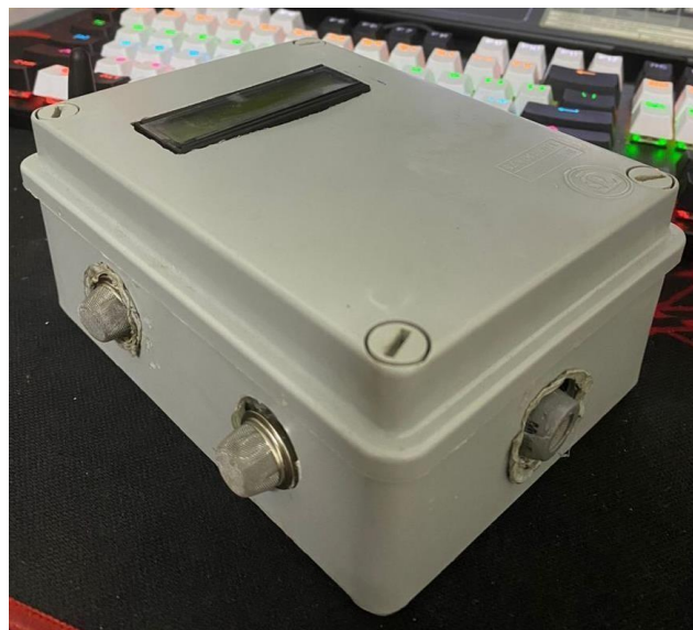
Fig. 17 AirGuardian: Real-Time IoT-Based Air Pollutant Monitor System device
