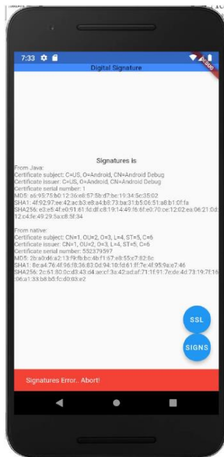
Figure 9 : Results of the interface if the Signature is invalid and SSL connection is secured
