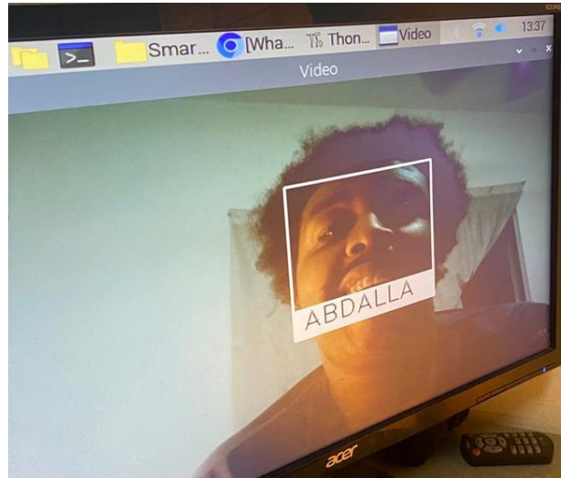
Figure 8: A face is detected using OpenCV and Face Recognition.
