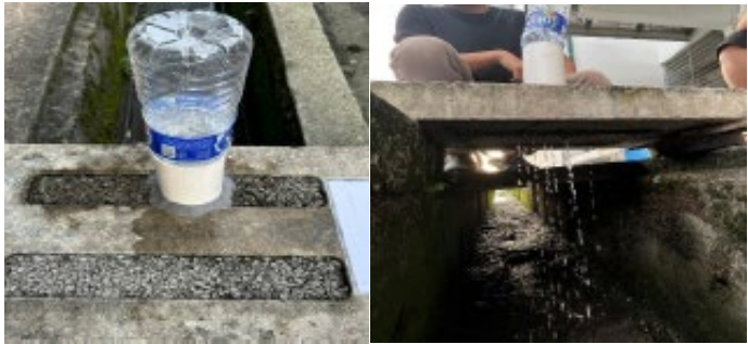
Figure 6.3: Infiltration ring on CPC slab by directly pouring 1.5L of water
