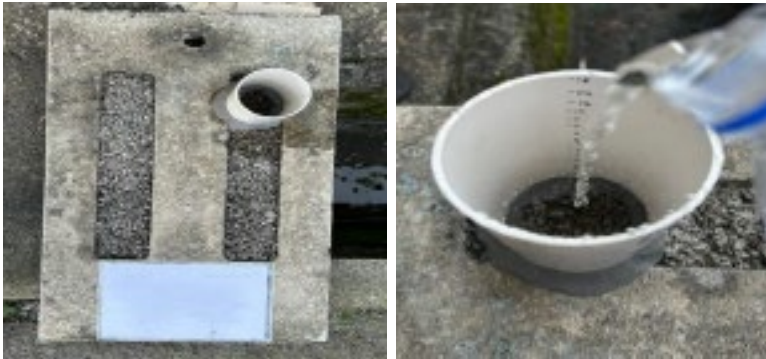
Figure 6.5: Infiltration ring test on CPC slab when poured with water of 12 cm depth
