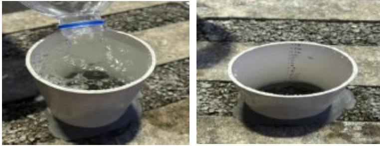
Figure 6.7: Infiltration ring test on CPC slab with measurements every 5 seconds
