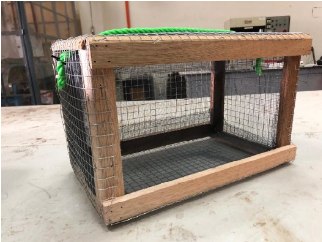
Figure 2.9: Tied the handle made up of nylon rope to the sampler
