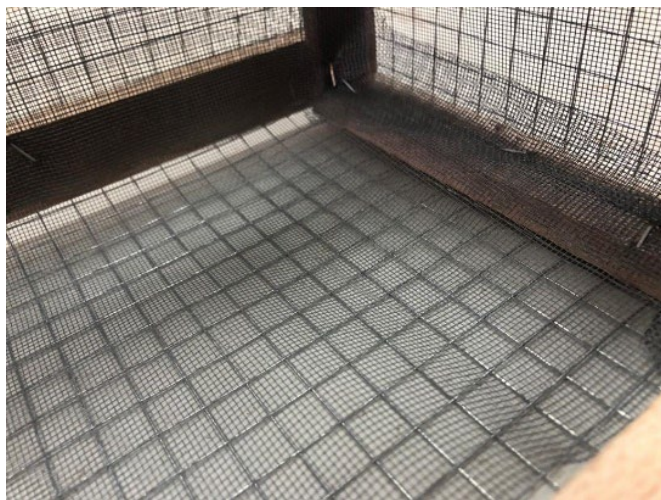
Figure 2.10: Install the wire mesh in the inner part of the sampler
