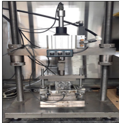
Fig. 3.4: Indirect Tensile Stiffness Modulus test setup.
