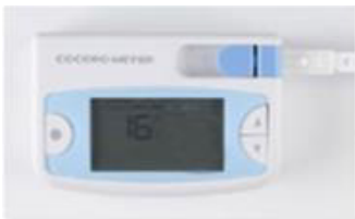
Figure 4.2: Kokorometer to measure salivary amilase level
