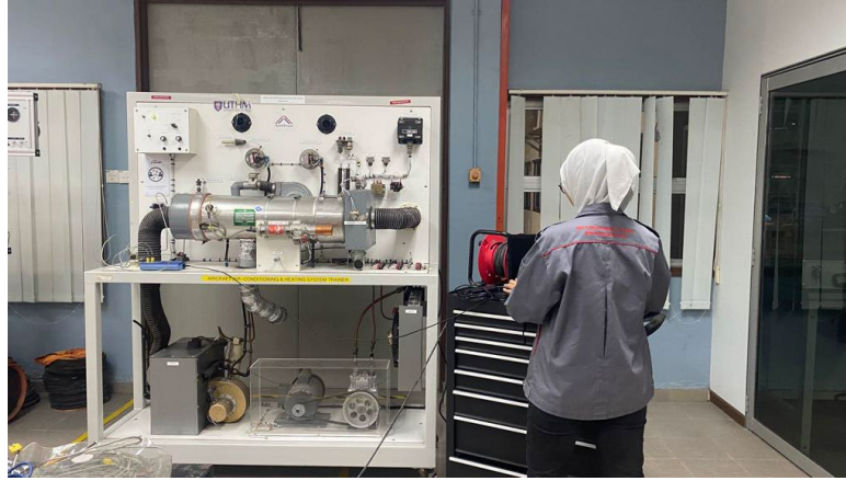
Fig. 3 - Temperature and relative humidity measurement of Model AS-43 heating system trainer
