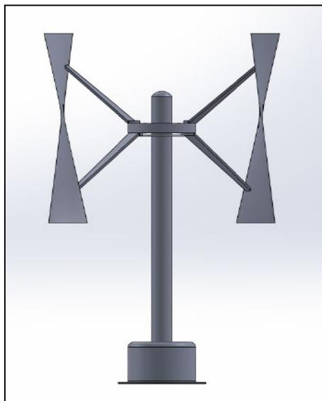
**Fig. 1 - Darrieus wind turbine with two-bladed model designed in SolidWork software**
