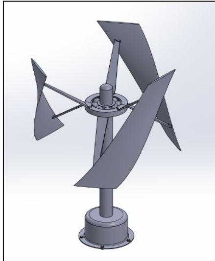
**Fig. 2 - Darrieus wind turbine with three-bladed model designed in SolidWork software**
