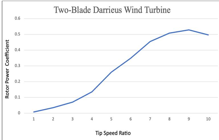
**Fig. 4 - Graph of rotor power coefficient against tip speed ration for two-bladed wind turbine**
