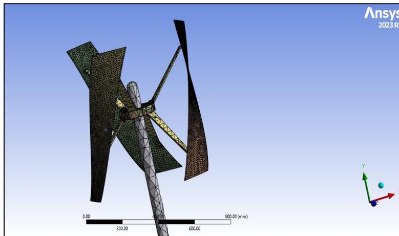
**Fig. 3 - Mesh generation for a wind turbine with three blades**
