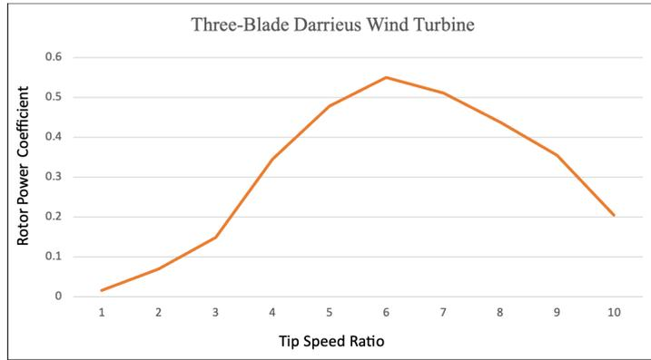
**Fig. 5 - Graph of rotor power coefficient against tip speed ratio for three-bladed wind turbine**
