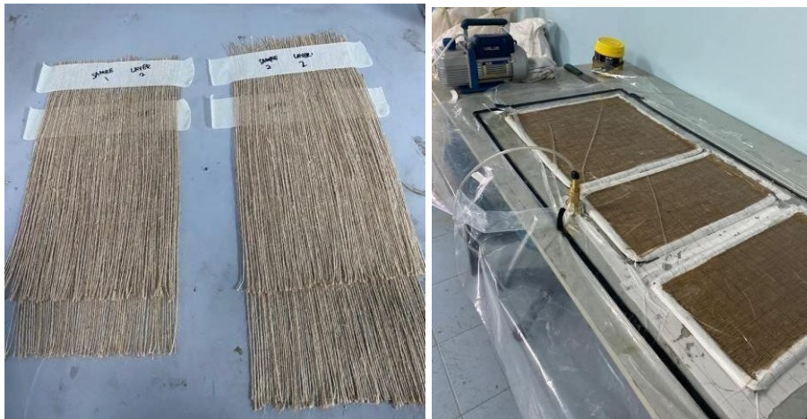
Fig. 3 - (a) Kenaf fiber preparation for vacuum bagging hand lay-up method; (b) hybrid composite fiber after vacuum bagging is applied and left to cure for 24 hours
