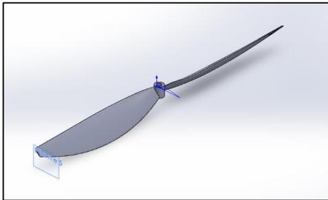
**Fig.1 - Propeller 1 without twisted blade**
