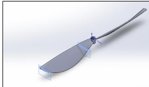
**Fig. 2 - Propeller 2 with twisted blade**
