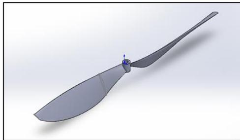
**Fig. 3 - Propeller 3 with twisted blade**
