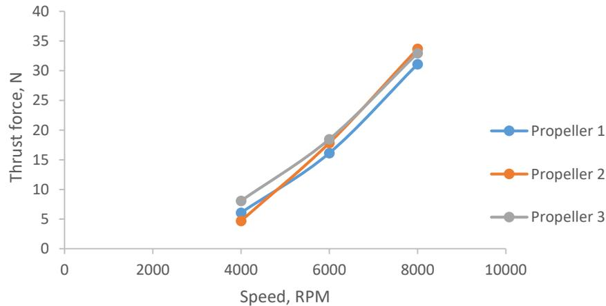
**Fig. 8 - Comparison of thrust force on Propeller 1, 2 and 3**
