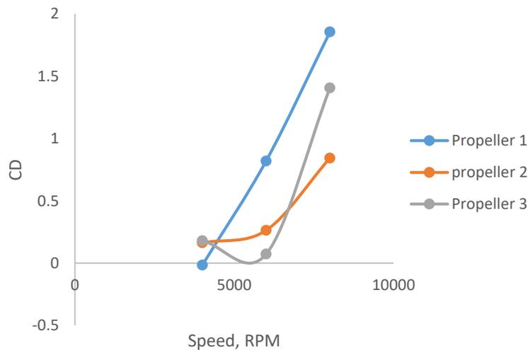
**Fig. 10 - Graph speed, RPM against  $C_D$  for all propeller**
