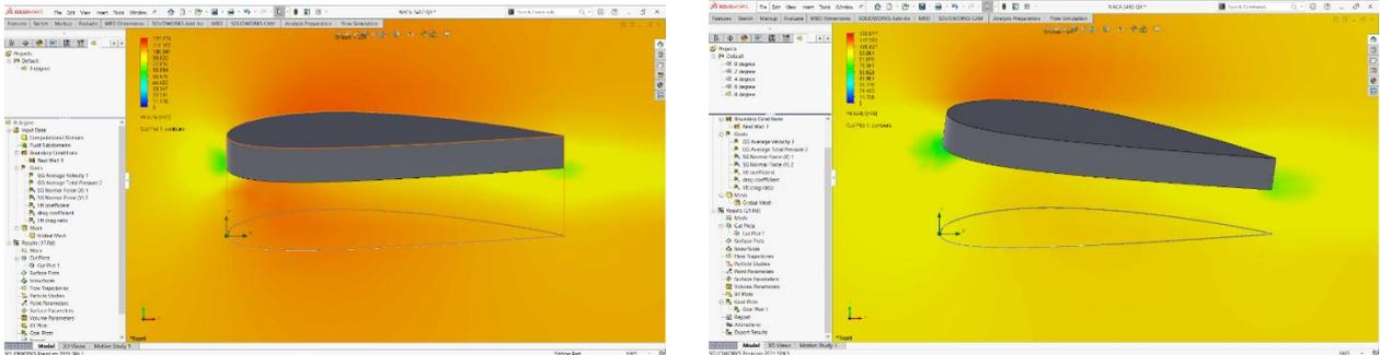
Fig. 5 - Velocity contour graph at 0° and 8° angle of attack at 0.3 m deflection
