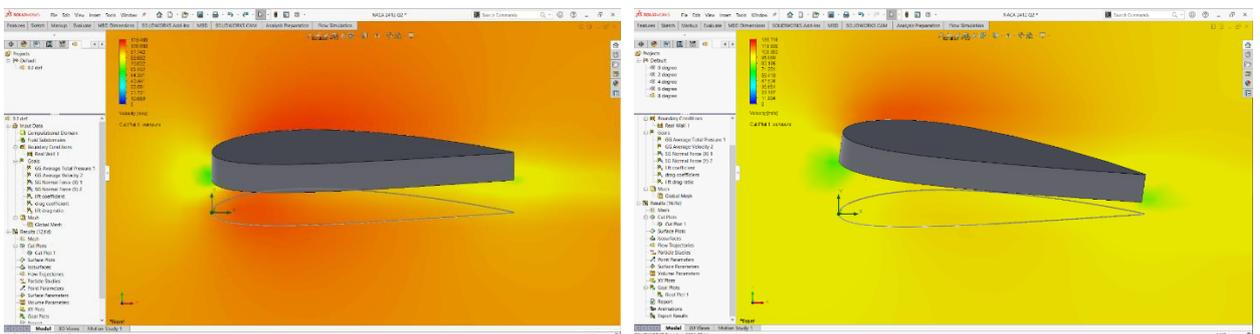
**Fig. 4 - Velocity contour graph at 0° and 8° angle of attack at 0.2m deflection**
