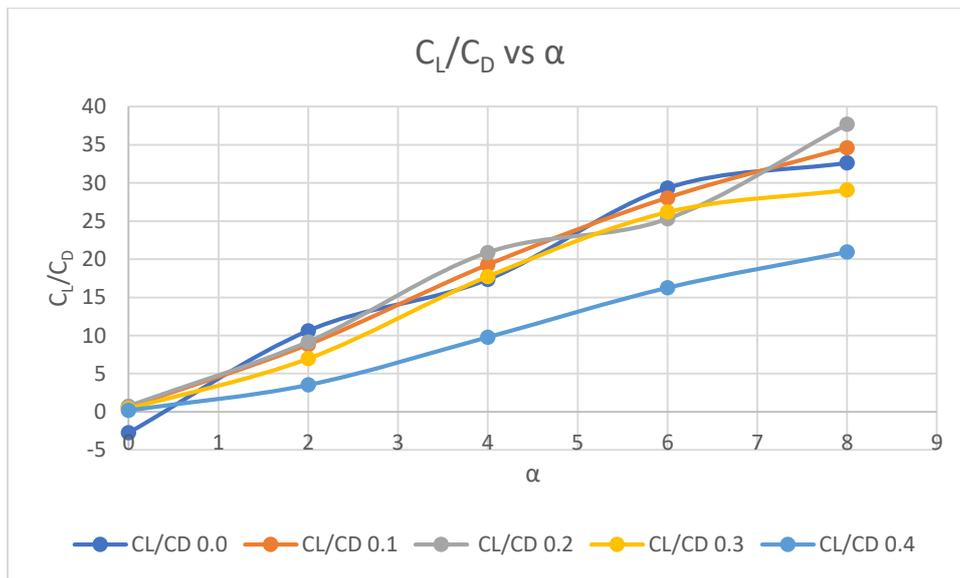
Fig. 8-  $C_L/C_D$  vs  $\alpha$  at 0° to 8° angle of attack
