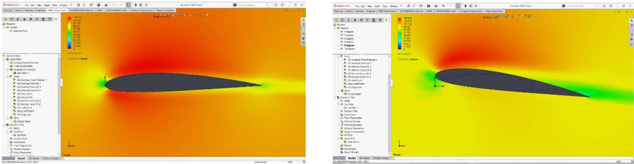
**Fig. 2 - Velocity contour graph at 0° and 8° angle of attack at normal configuration**
