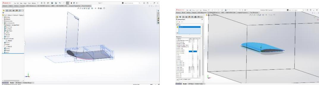
**Fig. 1 - (a)- airfoil deflection; (b) airfoil in a fluid domain**
