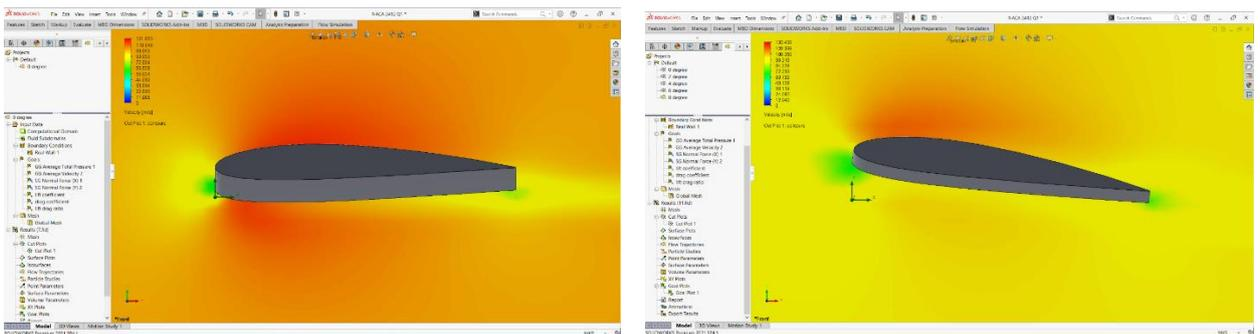
**Fig. 3 - Velocity contour graph at 0° and 8° angle of attack at 0.1m deflection**
