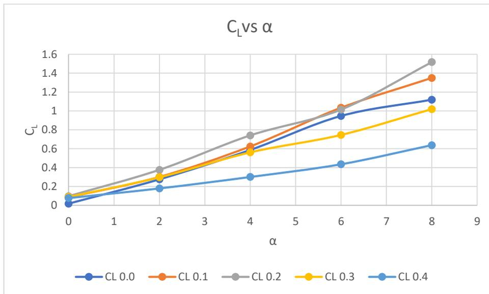
Fig. 7-  $C_L$  vs  $\alpha$  from 0° to 8° angle of attack
