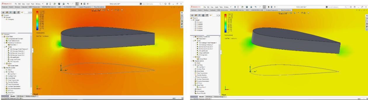
Fig. 6 - Velocity contour graph at 0° and 8° angle of attack at 0.4 m deflection
