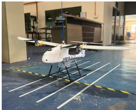
**Fig. 11 - Fully assembled Hybrid VTOL Fixed-Wing Drone**
