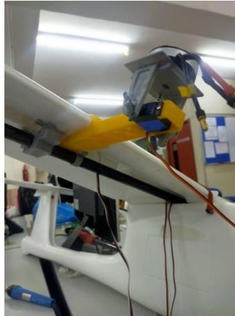
**Fig. 10 - Upper part of tilting mechanism connected to wing**
