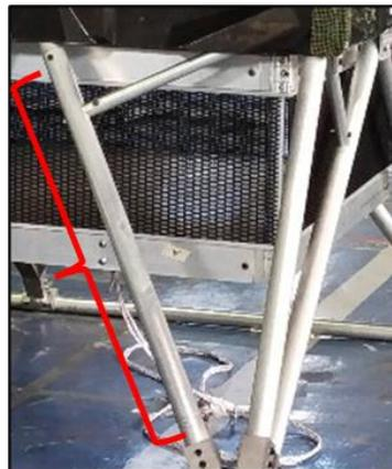
**Fig. 2 - The landing gear of C-Drone UTHM labelled in red**
