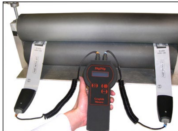
Fig. 6 - Profiling pressure film application
