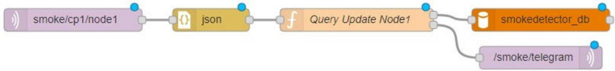
Fig. 8 - Flow-based programming tool using Node-RED software for SN1
