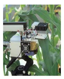
Fig. 3 - Picture showing the leaf gas exchange measurement with the 6400-02B LED light source.
