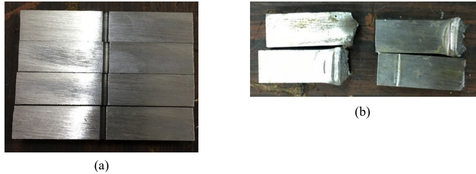
Fig. 12 - Test coupon (a) before and; (b) after Charpy Impact Test
