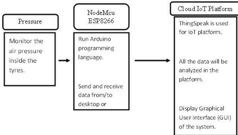
Fig. 2 - CTAPMS block diagram
