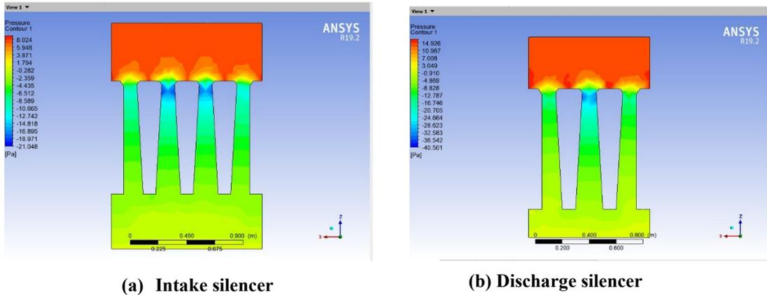
**Fig. 6 - Pressure contour for discharge silencer and intake silencer**
