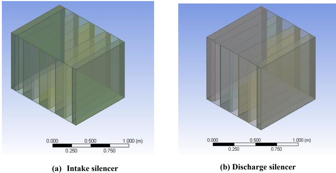
Fig. 2 - Geometry model of discharge silencer and intake silencer
