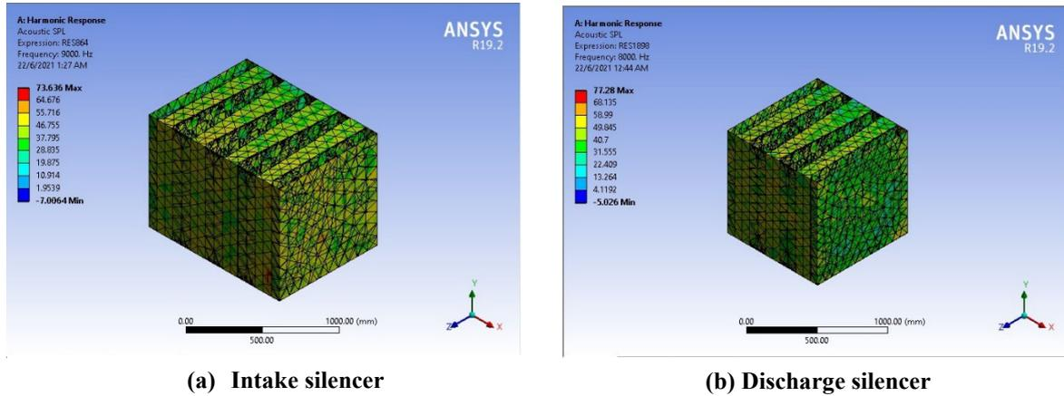
Fig. 8 - SPL contour for discharge silencer and intake silencer
