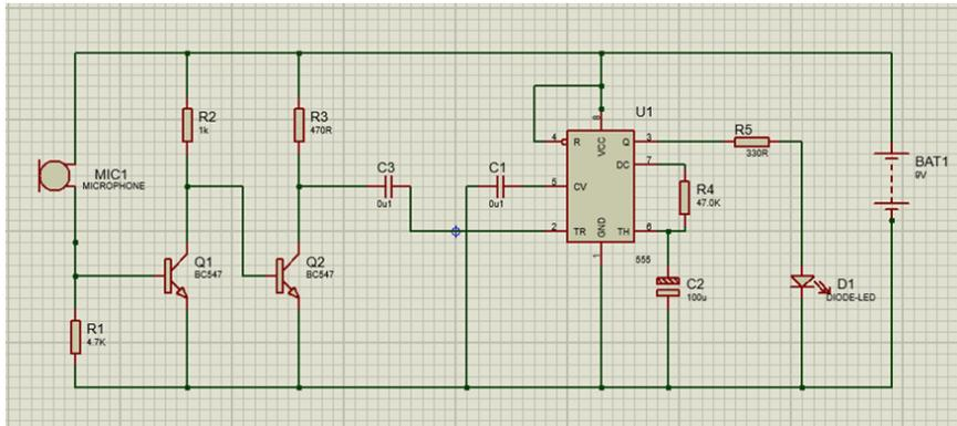
**Fig. 1 - The circuit diagram that has been drawn using the Proteus software**
