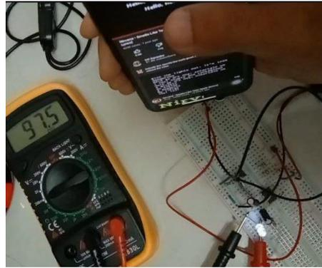
**Fig. 4 - Measuring the output voltage for iPhone speaker as the source of sound energy**
