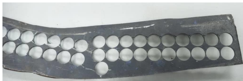
Fig. 1 – Raw 22MnB5 in the form of grinded steel
