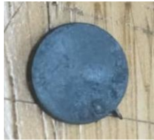
Fig. 3 – 22MnB5 after cut by laser cutting machine
