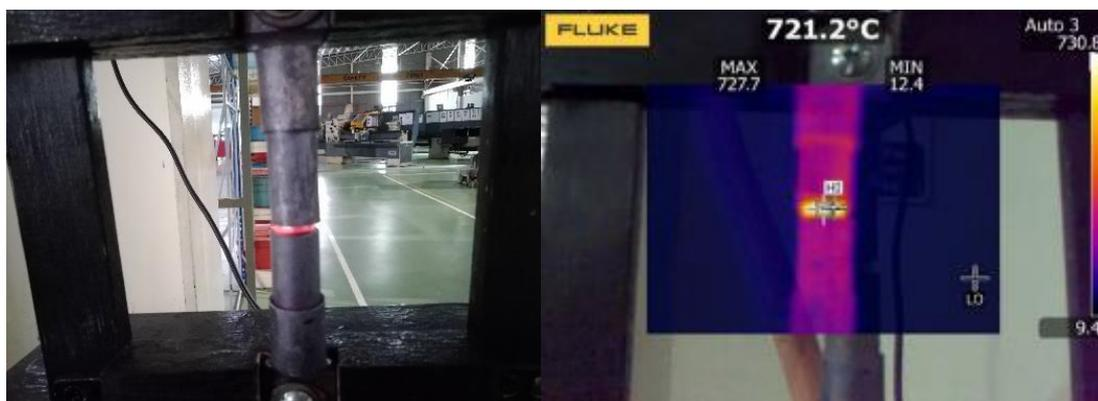
**Fig. 6 - The specimen was being test and sinter using the machine x at 7 minutes, the temperature achieves 721.2°C**
