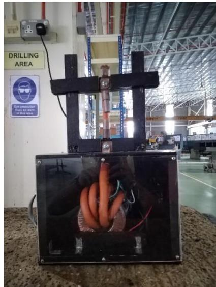
**Fig. 5 - Resistance sintering furnace machine prototype**
