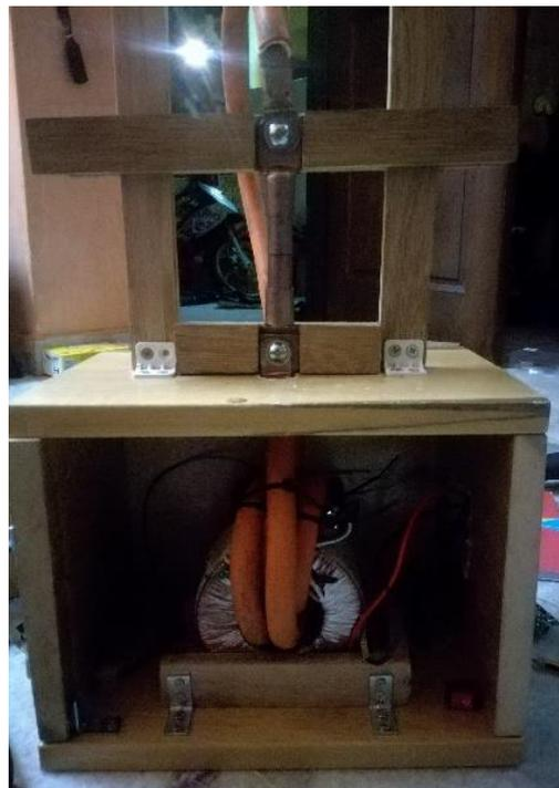
Fig. 4 - Resistance sintering furnace after done assembly process
