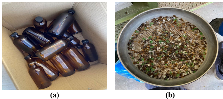
Fig. 1 (a) Glass waste before crush; (b) Glass waster after crush
