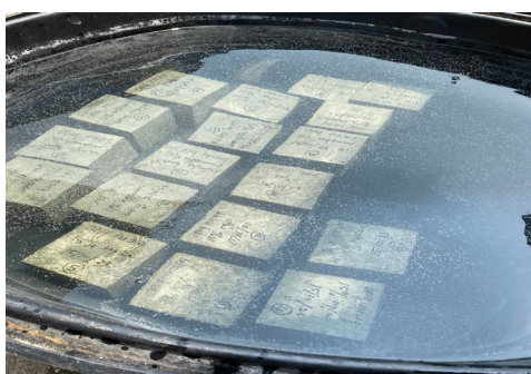
Fig. 3 Concrete curing process
