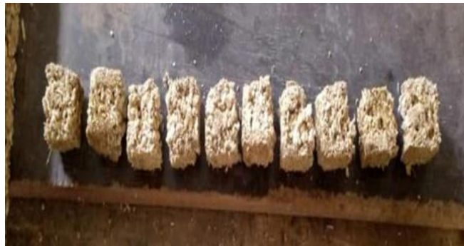
Fig. 7 Density and moisture content test samples
