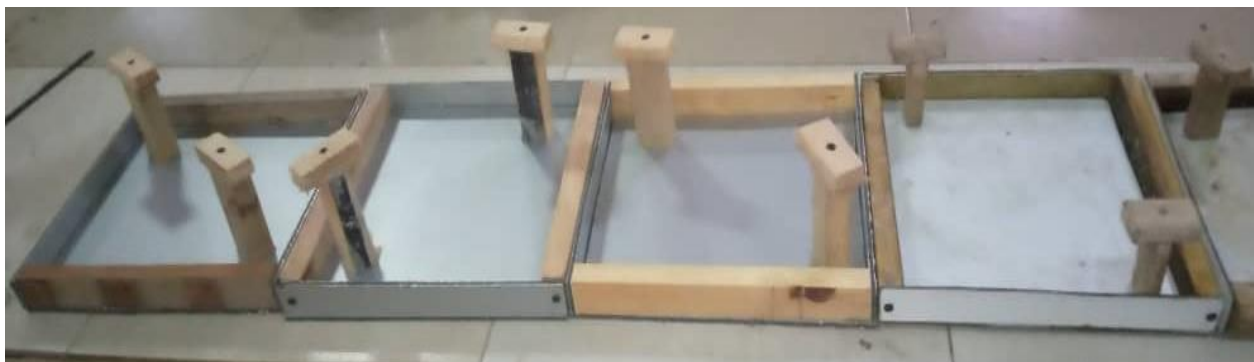
Fig. 5 Aluminium mold boxes for particleboard pressing
