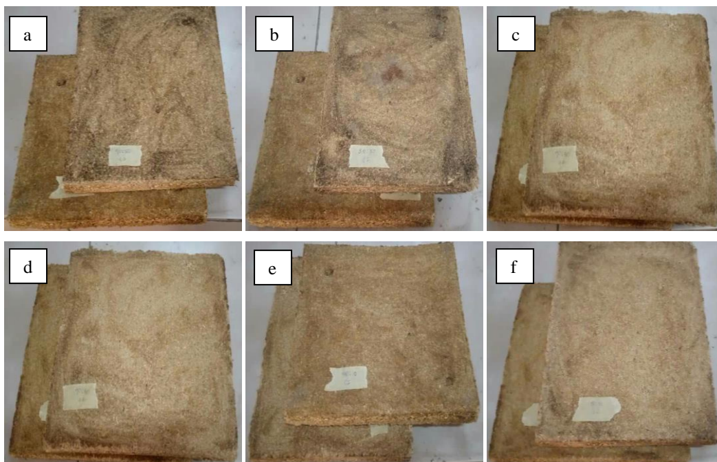
Fig. 6 Particleboards produced and their ratios; (a) 90:10 mix ratio; cassava starch; (b) 70:30 mix ratio; cassava starch; (c) 50:50 mix ratio; cassava starch; (d) 90:10 mix ratio; urea formaldehyde; (e) 70:30 mix ratio; urea formaldehyde; and (f) 50:50 mix ratio; urea formaldehyde
