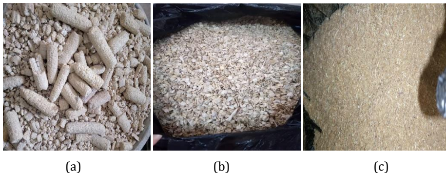
Fig. 2 Corn cob particles; (a) CC ready to be crushed; (b) >1mm CC particles; (c) < 1mm CC particles
