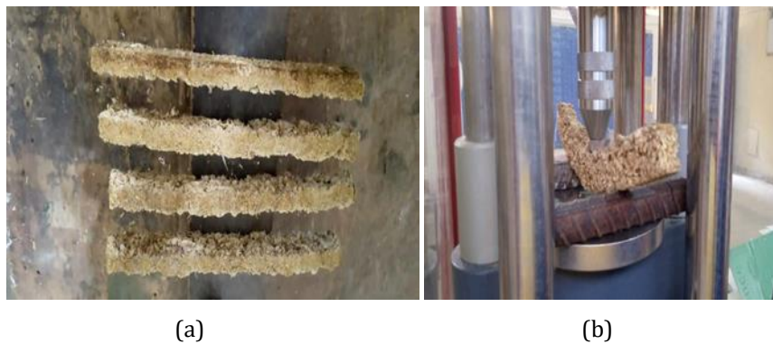
Fig. 9 Mechanical testing samples and test set-up; (a) MOR and MOE test samples. And (b) test setup
