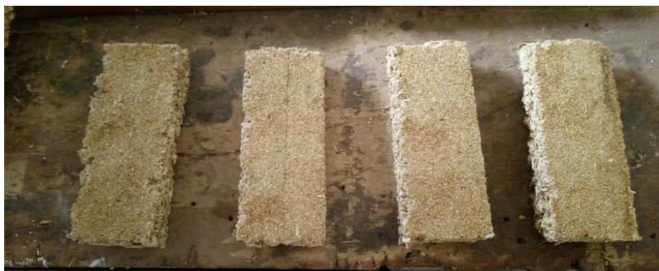
Fig. 8 Thickness swelling and water absorption test samples
