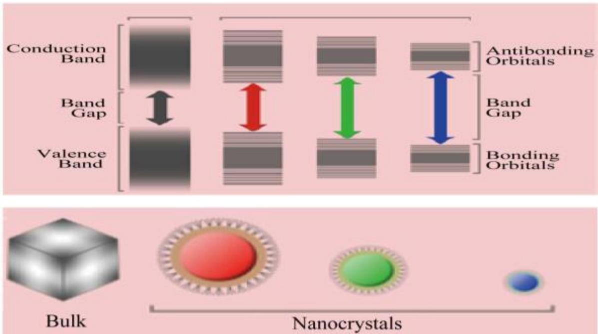
Fig. 1 Schematic energy band diagram of nanocrystal-line CdSe and bulk materials [10]
