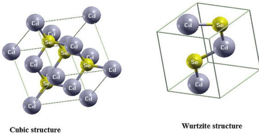
Fig. 2 Geometrical structure for CdSe nanomaterials for different phases Cubic and Wurtzite structures [12]
