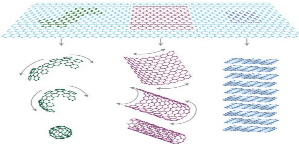
**Fig. 3** Mother of graphene form (fullerene, carbon nanotubes and graphite) [19]
