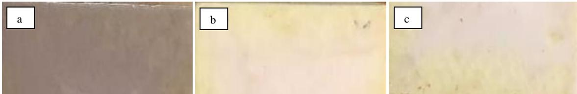
Fig. 2 - Ca-Al<sub>2</sub>O<sub>3</sub> polymer-based radiation shielding composites (a) Ca from snail shells; (b) Ca from periwinkle shells, and; (c) Ca from seashells
