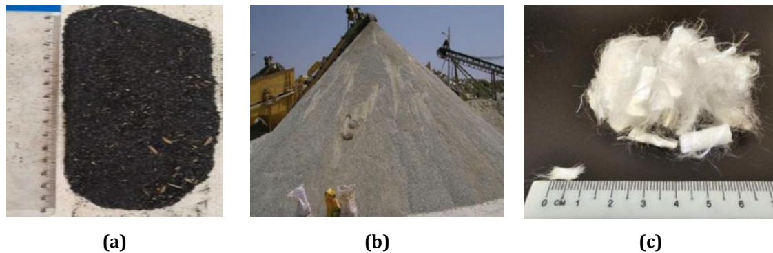
Fig. 1 Sustainable material used in this study as (a) Rice husk ash; (b) Quarry dust; and (c) Polypropylene fiber
