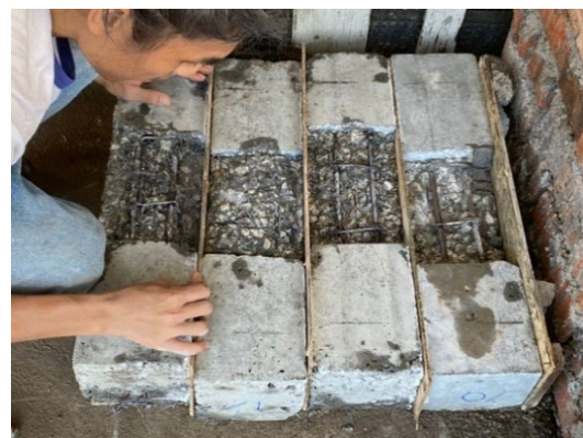
Fig. 5 Remolding defect beams
