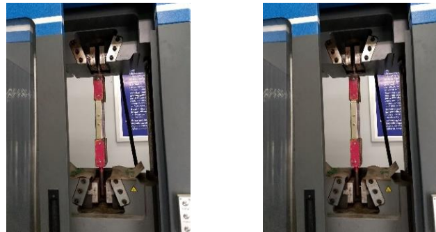
Fig. 2 Sample placement at UTM machine
