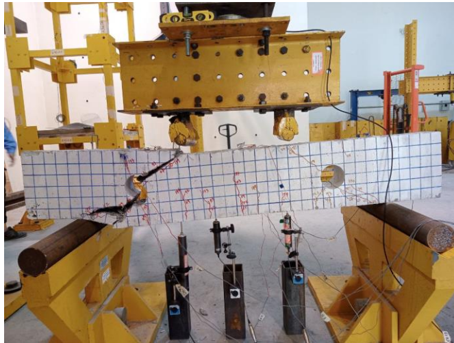
Fig. 10 - Crack pattern of beam BO-1-RSFM
