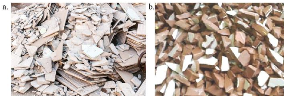
Fig. 2 - (a) ceramic tiles waste on site; (b) ceramic tiles waste after crushing
