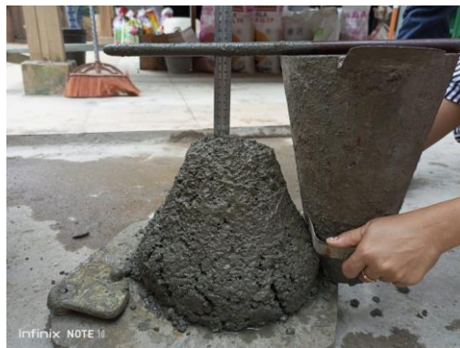
Fig. 1 - Slump test of concrete with 10% bottom ash
