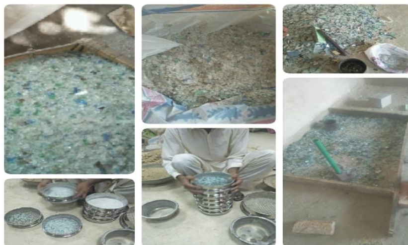
Fig. 1 - Preparation of fine aggregates through glass waste
