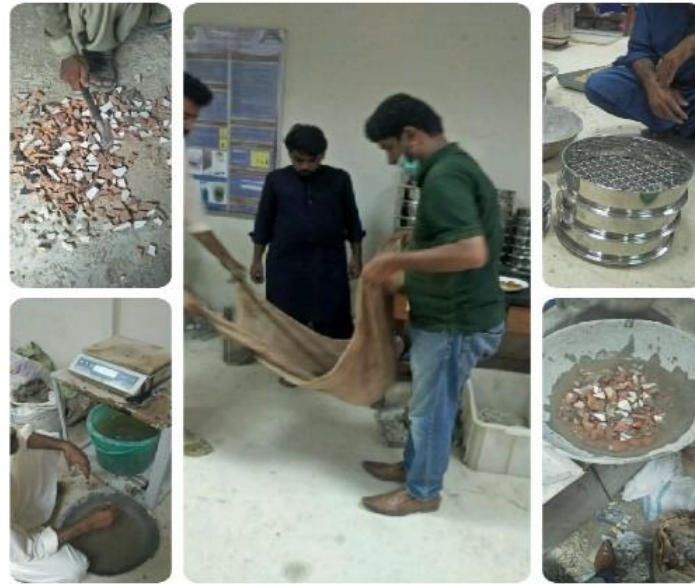
Fig. 2 - Preparation of coarse aggregates through ceramic tile waste
