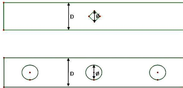
**Fig. 2 - Dimension of web openings**
