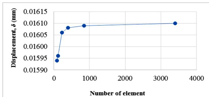
Fig. 5 - Graph of displacement against number of elements
