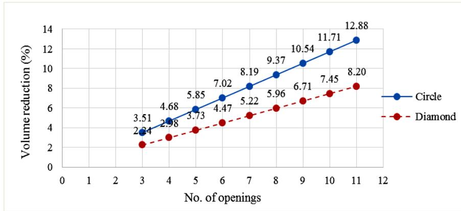
**Fig. 11 - Percentage of volume reduction against no. of openings and different opening shapes with 50 mm edge distance**
