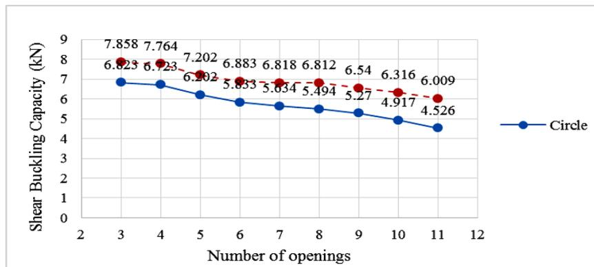
**Fig. 12 - Shear buckling capacity against no. of openings and opening shape with 50 mm edge distance**
