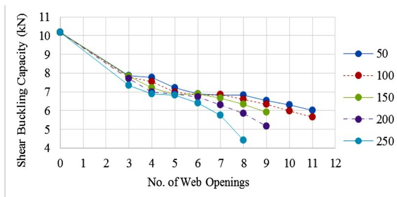
**Fig. 8 - Shear buckling capacity of Lysaght plain channel against no. of diamond openings with different edge elements**
