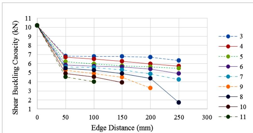
**Fig. 10 - Shear buckling capacity against no. of circle openings with different edge distance**
