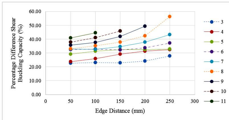
**Fig. 9 - Trend of plain channel section with a number of diamond openings and different edge distance**
