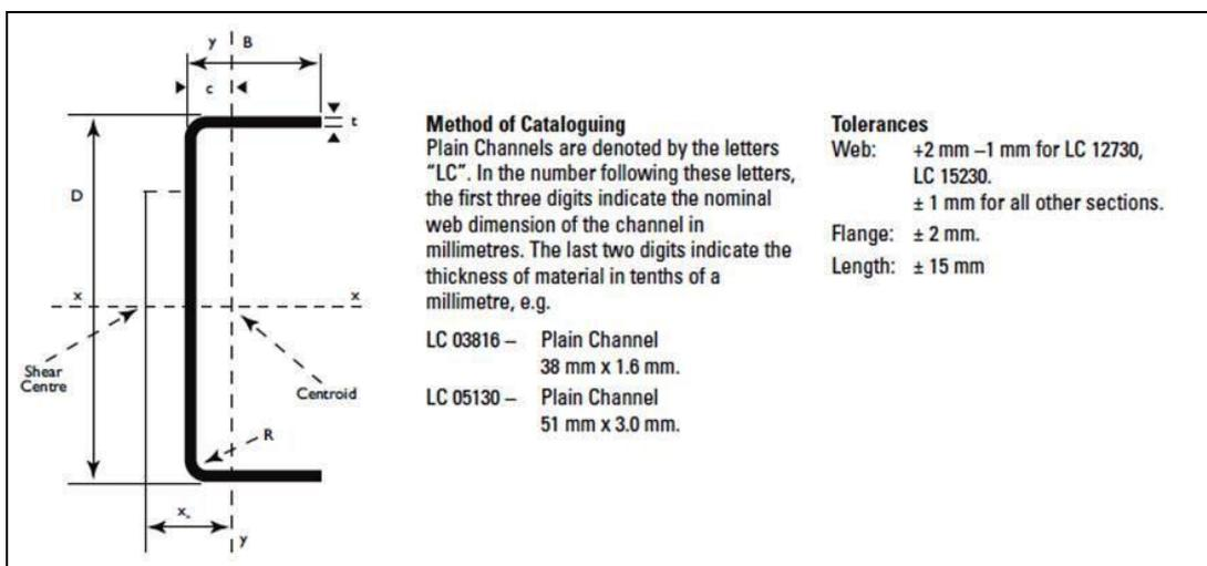
Fig. 1 - Dimension view of cold-formed plain channel steel section
