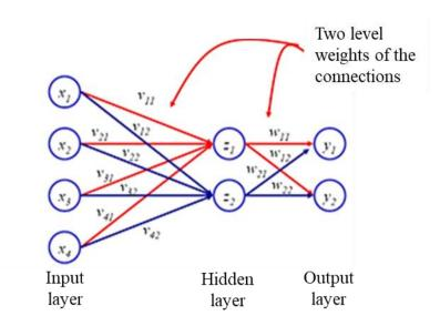
Fig. 3 - Multi-layer neural network architecture.
