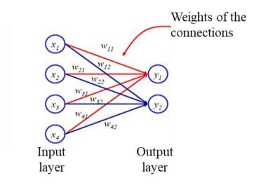
Fig. 2 - One-level neural network architecture.
