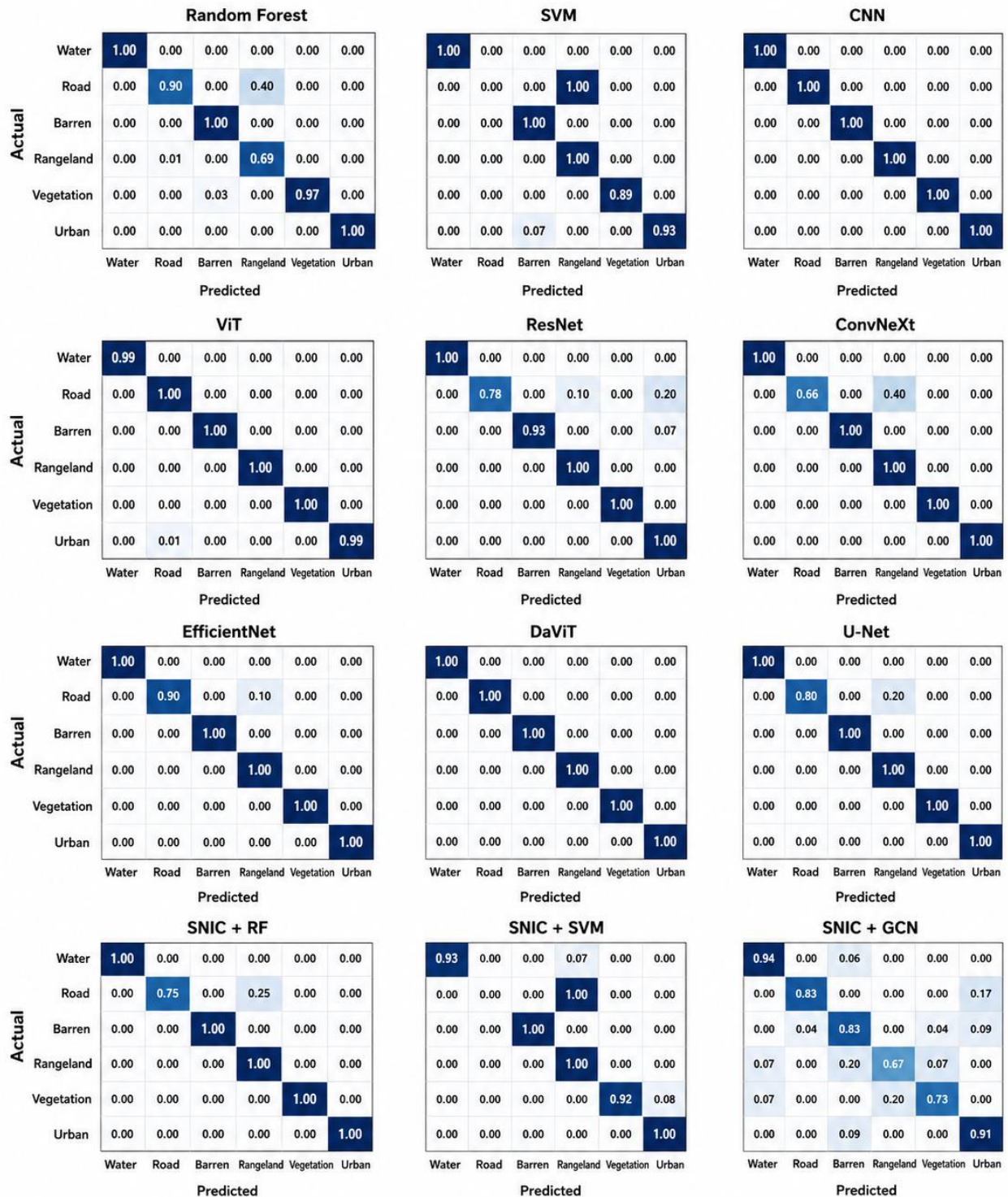
Fig. 6 Confusion matrices that are normalized for each of the twelve classification models. For each class, the values show the percentage of reference samples that were correctly or incorrectly classified. Higher values are indicated by darker hues
