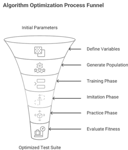
Fig. 2 Optimization process for implementation of STBO for T-Way test suite generation
