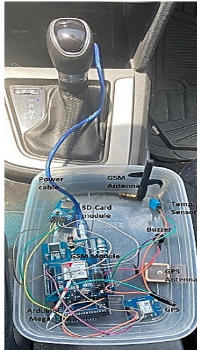
Fig. 1 Hardware setup of the proposed system installed inside the car, powered from the built in USB port
