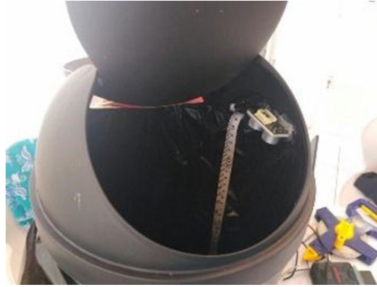
Fig. 3 Placement of ultrasonic sensors for measuring the height of the trash heap
