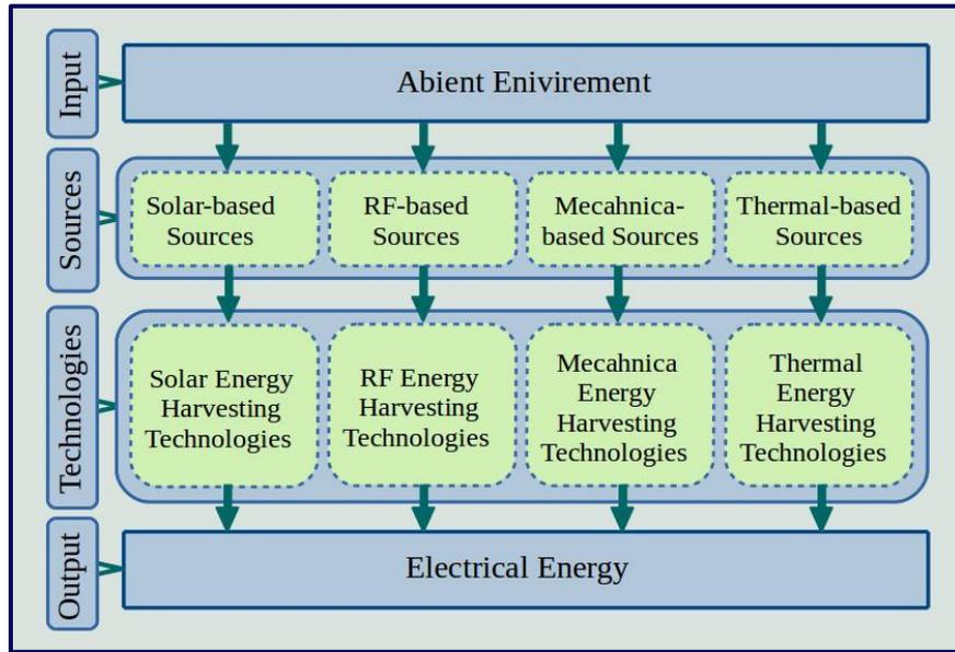
Fig. 3 - Ambient energy-harvesting sources for IoT-based wireless nodes
