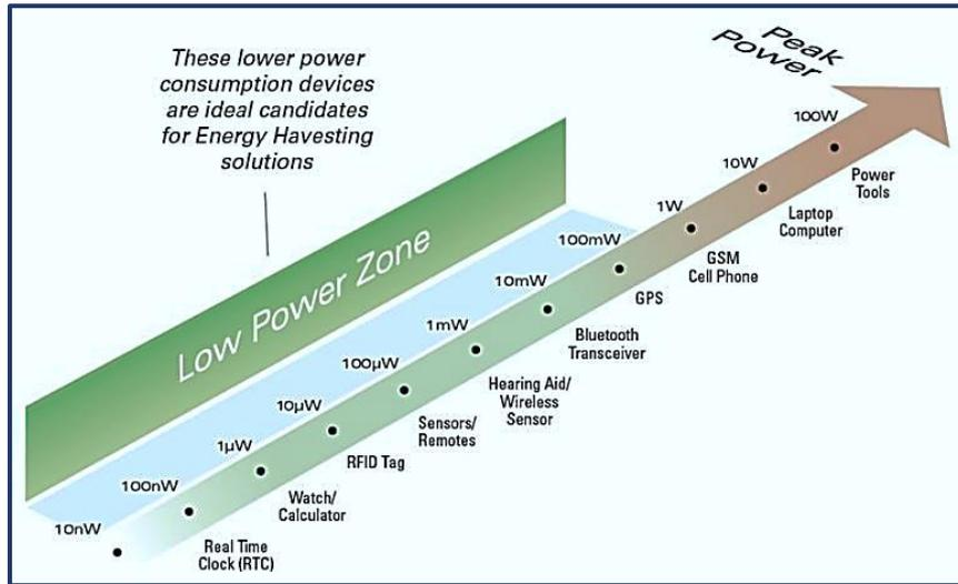
Fig. 5 - Peak Power Levels for Typical IoT Devices (Source: [55])
