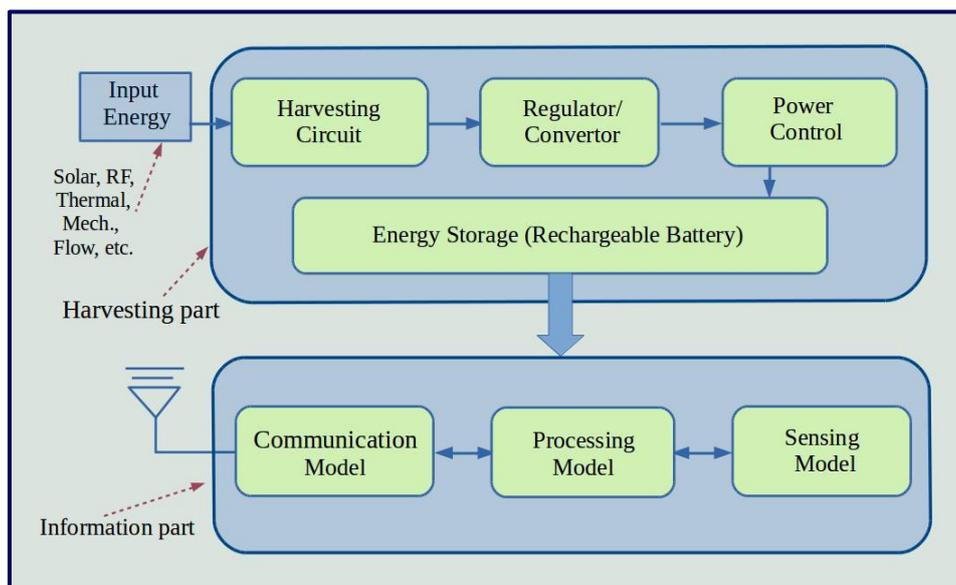
Fig. 4 - A general architecture of the energy-harvesting node
