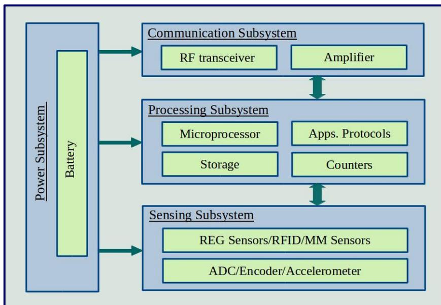
**Fig. 1 - A general architecture of the IoT-based wireless node**
