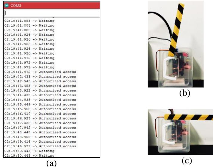
**Fig 4 - (a) Serial monitor display for barrier gate status; (b) Barrier gate when tag is detected; (c) Barrier gate when no tag is detected.**
