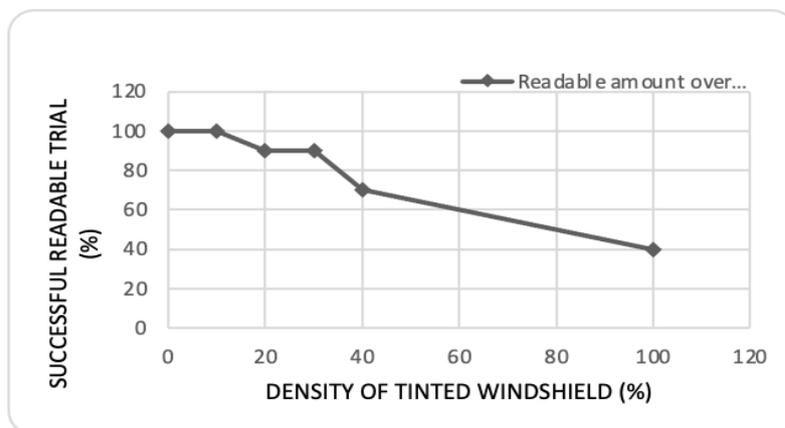
**Fig 5 - Readability of tag in various density of tinted windshield in day time**
