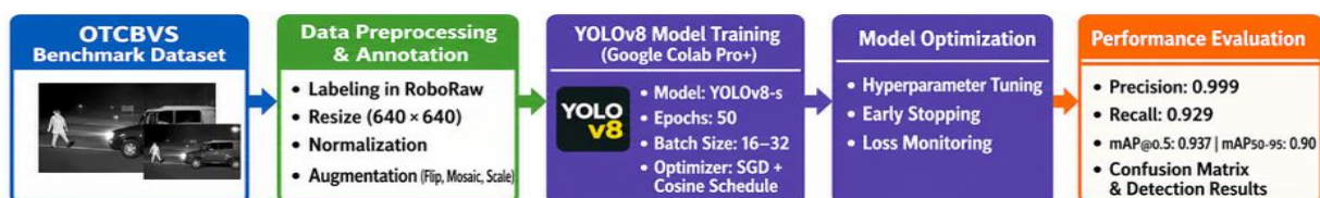
Fig. 1 Workflow of the proposed YOLOv8-based infrared intrusion detection and classification framework
