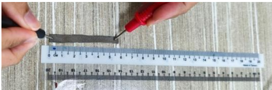
Fig. 9 Resistance testing using multimeter
