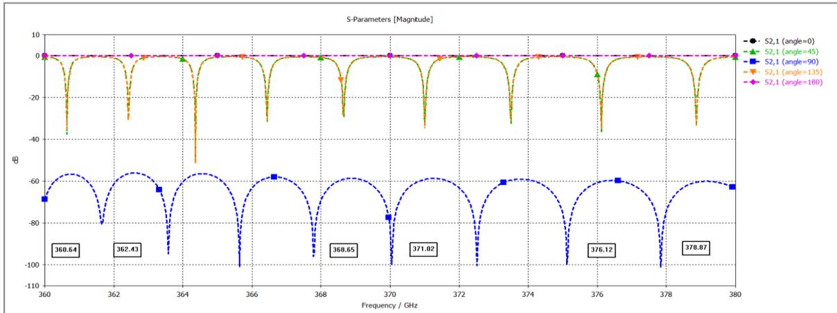
**Fig. 3 - The insertion loss (S21, dB) with different polarization angle, 0°, 45°, 90°, 135°, 180° at port 2 from 360 GHz to 380 GHz**
