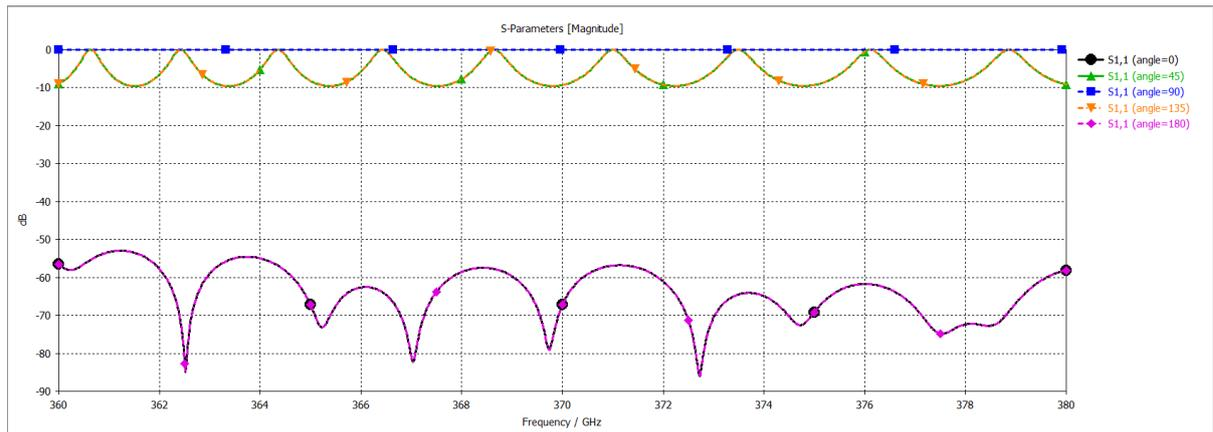
**Fig. 2 - The return loss (S11, dB) at port 1 with different polarization angle, 0°, 45°, 90°, 135°, 180° at port 2 from 360 GHz to 380 GHz**
