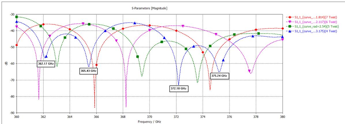
**Fig. 4 - The return loss, (S11, dB) of the waveguide at different twisting rate**
