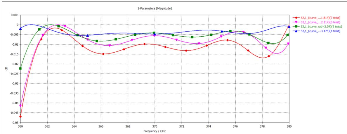
**Fig. 5 - The insertion loss, (S21, dB) of circular waveguide with different twisting rates**
