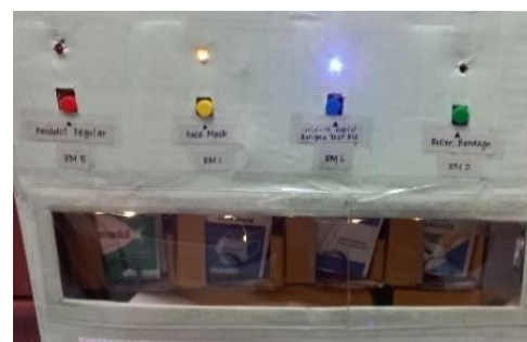
Fig. 13 - Current state of all LEDs when face mask and rapid antigen test kit is chosen
