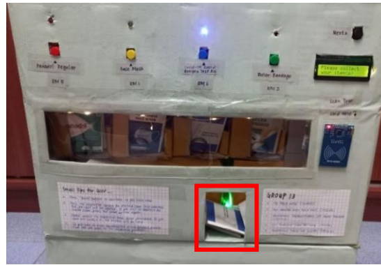
Fig. 14 - The item is vended to the “item collecting slot”
