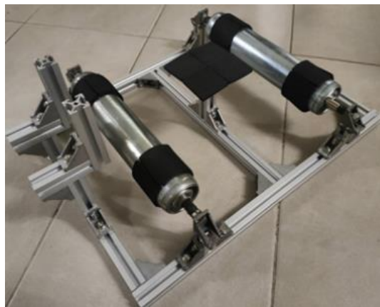
Fig. 6 - Complete chassis dynamometer
