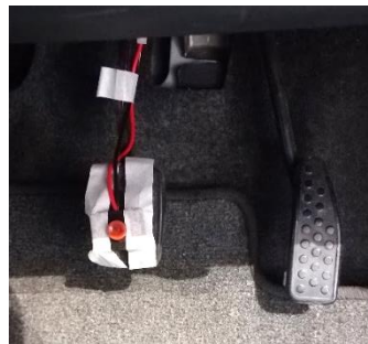
Fig. 2.4 - Push button attached to the brake pedal
