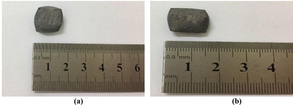
**Fig. 8 - Macroscopic images of the Al (LM6) alloys after heated at the temperatures of (a) 700°C; (b) 750°C for 30 min**
