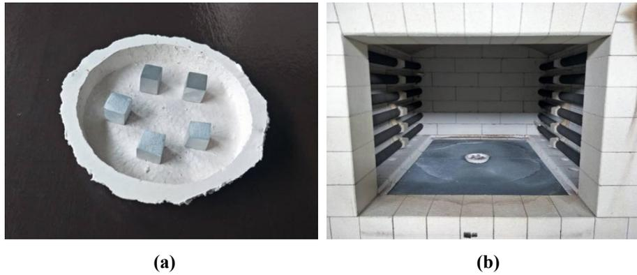
Fig. 6 - (a) Al alloy cubes charged into investment casting ceramic plate; (b) loading samples at the middle of the laboratory furnace
